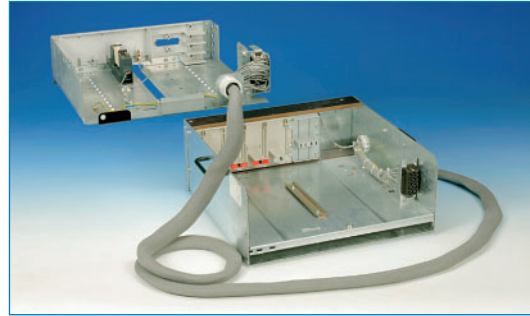
Test unit for testing withdrawable motor/feeder units outside the MCC.
